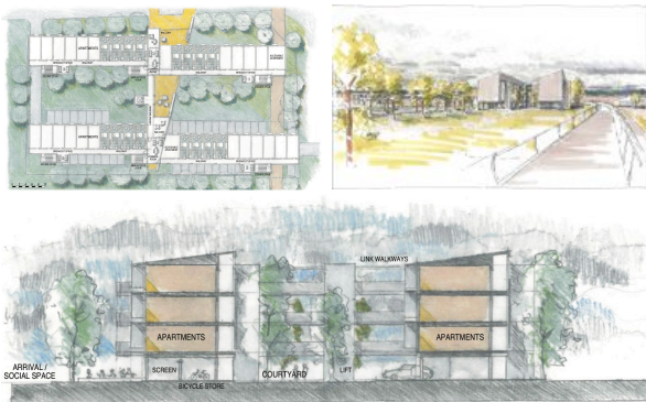
Figure 1. NRAS Inveresk preliminary proposal: Top – Site Plan and perspective view. Bottom – Section. Image credits. Morrison & Breytenbach Architects
