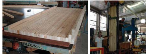
Figure 8: Full scale prototype (left). The author with prototype panel being prepared for load testing (right)
