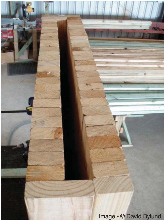
Figure 2.21 Prototype GPLT panels in truss and frame manufacturer's factory. Photograph by D.Bylund
