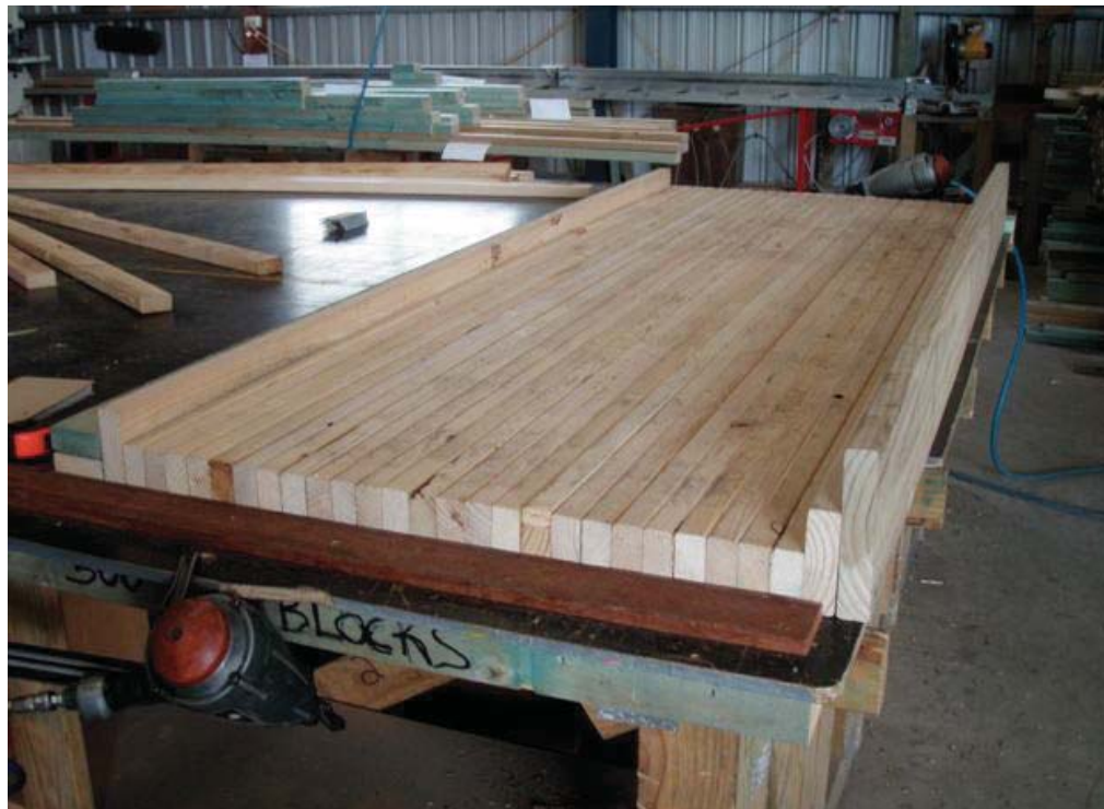
Figure 2.20 Prototype GPLT panel in truss and frame manufacturer's factory. Photograph by D.Bylund
