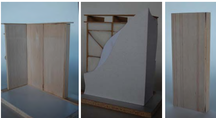
Figure 2.2 1:10 scale GPLT Panels and wall element cutaway models. Images: D.Bylund
