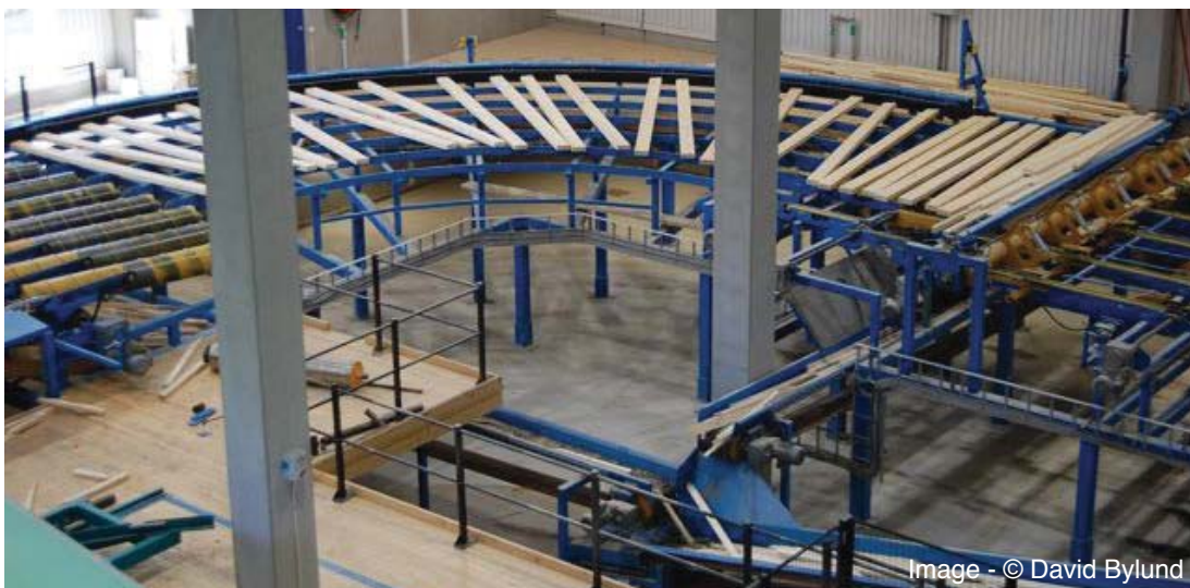
Figure 2.23 Modern sawmilling operation in Sweden preparing timber for finger jointing and lamination. Photograph by D.Bylund
