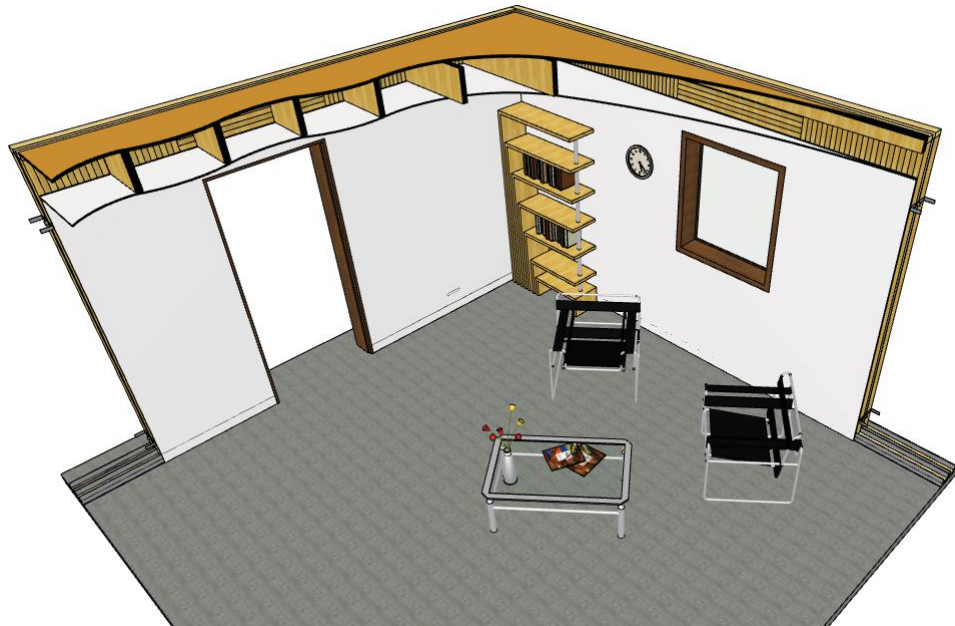
Figure 3.4 Cutaway of completed ground floor walls showing slab, walls with internal lining and timber floor structure above.
