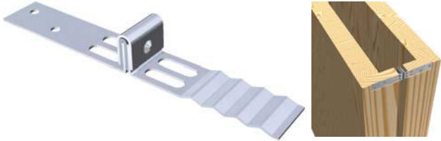
Figure 2.13 Off-the-shelf Resilient Wall Tie (MB01GA), (left) and wall tie in position (right) by Matrix Industries Pty Ltd. This system proved to be unfeasible because the fixings required access to an internal face of the 120mm x 35mm end trimmer.
