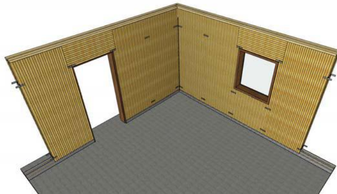
Figure 3.13 Corner panel assembly including openings
